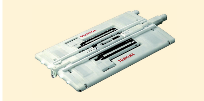
Inspection robot for turbine generators
