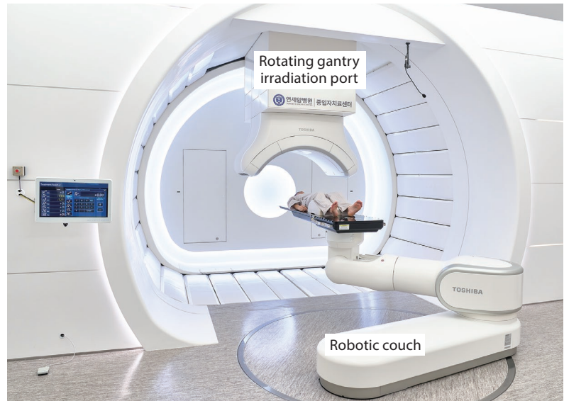
Rotating gantry irradiation room
