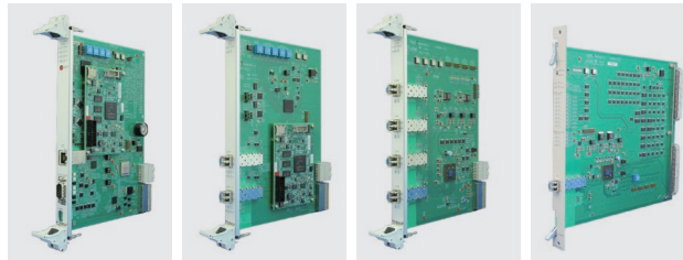
Printed circuit boards in digital controller
