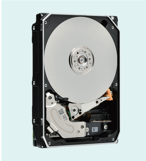
Prototype HDD featuring storage capacity exceeding 30 TB
