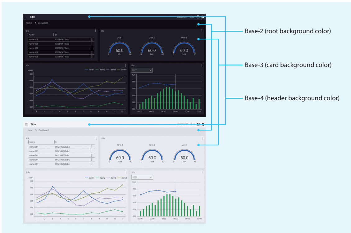
Example of design tokens using base colors specified by TOSHIBA SPINEX Design System
