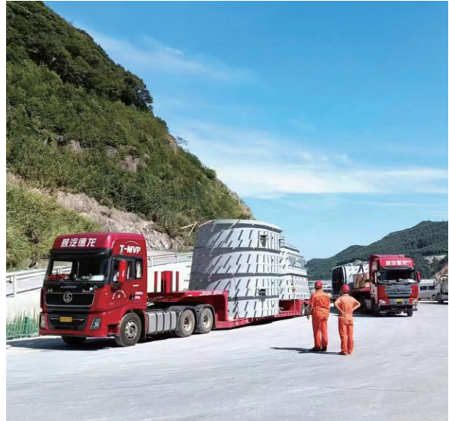
Shipment of draft tube for Unit 1
