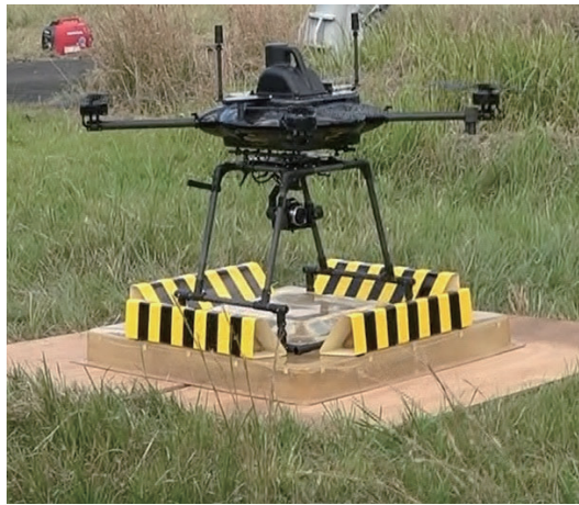
Low-profile inductive charging port and drone with wireless charger
