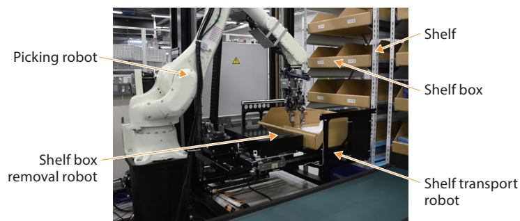
Picking operation in picking robot work area
