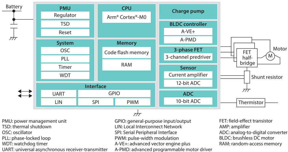
**Architecture of SmartMCD integrated motor control driver for automotive applications**
