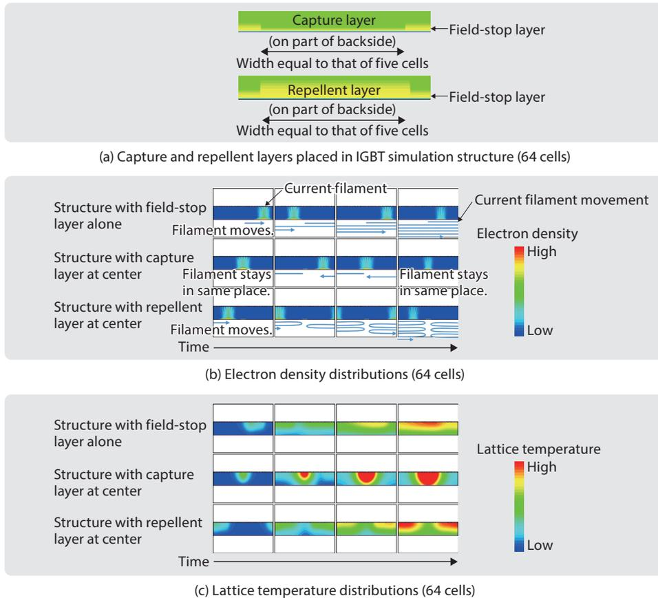
Results of simulations of current filament behavior depending on device structure of IGBTs
