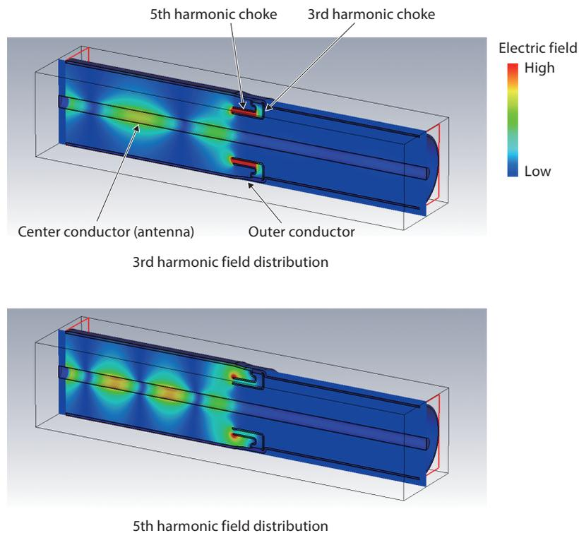
**Result of simulation using optimization tool at harmonic suppression choke structure design stage**
