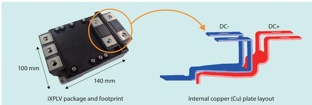
iXPLV package for SiC MOSFETs and internal structure of electrodes
