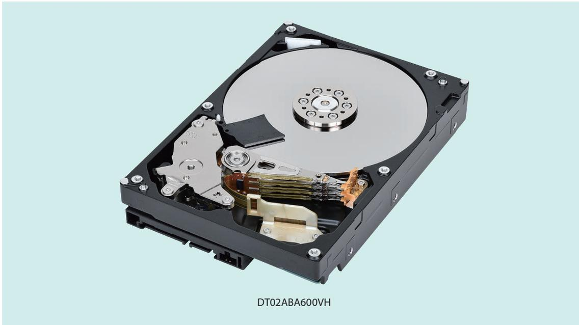
6 Tbyte 3.5-inch SMR HDD for surveillance camera systems
