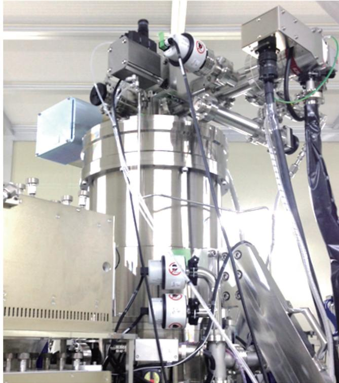
MBM™-2000 mask writer using multiple electron beams
