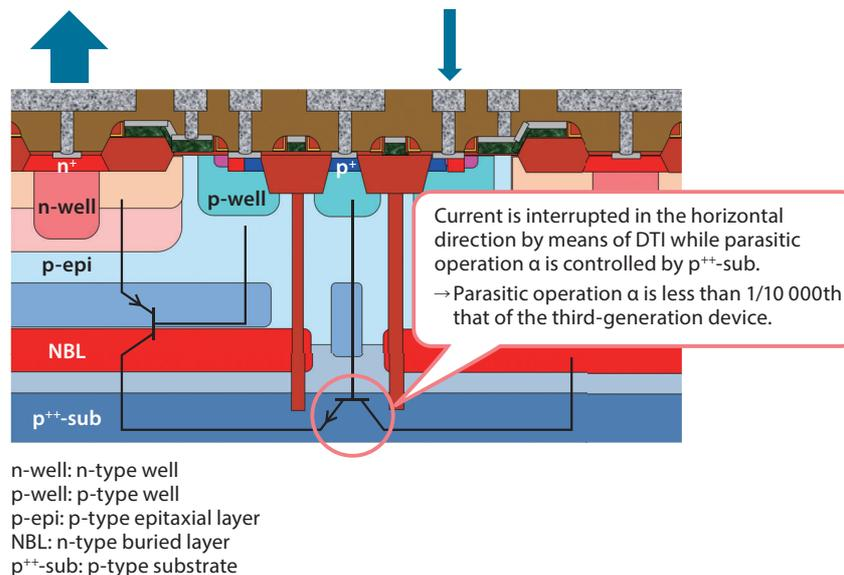
Cross-sectional structure of fourth-generation analog power IC
