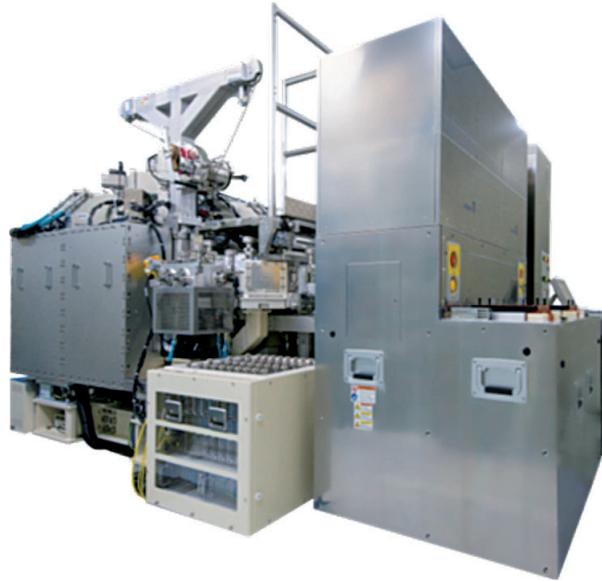
EBM-9500PLUS/EBM-8000P electron beam mask writer
