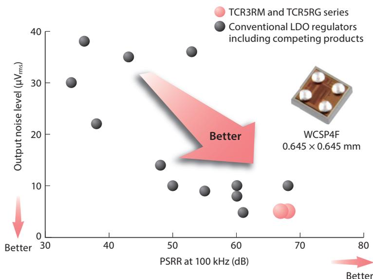
Lower noise and higher PSRR achieved by TCR3RM series and TCR5RG series linear regulator ICs for image sensors compared with conventional products
