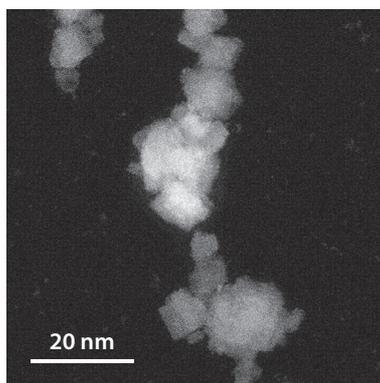
Transmission electron microscope (TEM) image of  $\text{WO}_3$  nanoparticles
