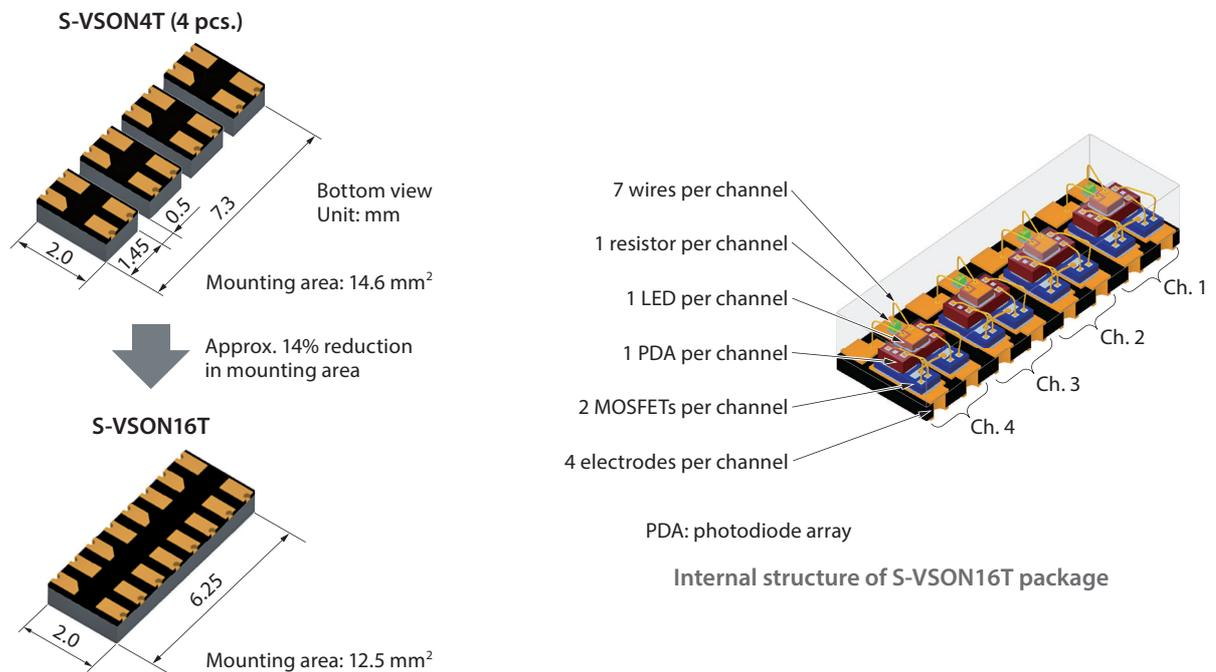
Comparison of photorelay mounting area when using four S-VSON4T packages and S-VSON16T package
