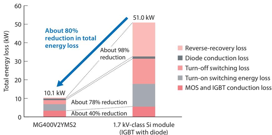
Calculated using data simulated at a channel temperature of 150°C
