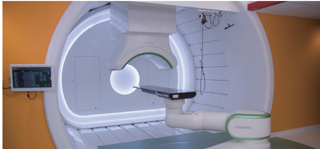
Treatment room equipped with downsized superconducting rotating gantry at East Japan Heavy Ion Center, Faculty of Medicine, Yamagata University
