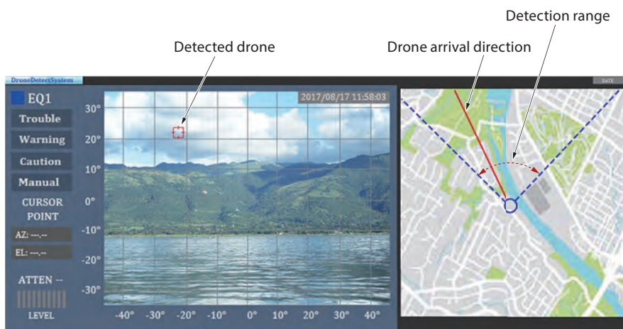
Example of monitoring control terminal display
