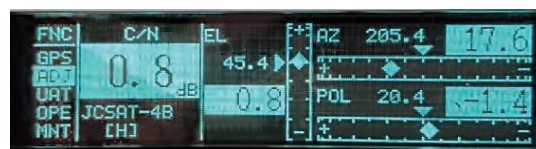
Example of display supporting satellite look-angle adjustment
