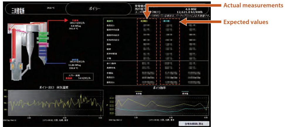
Example of plant performance monitoring display
