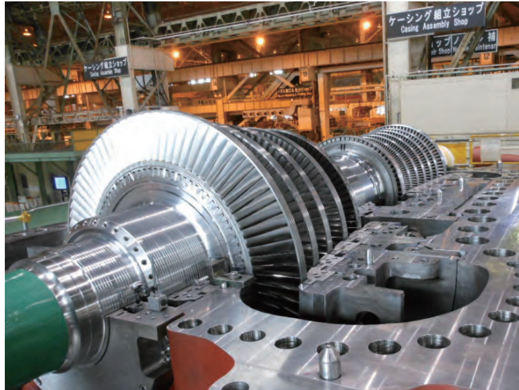
HIP turbine under assembly for Shin-Onoda Thermal Power Station Unit 2 of The Chugoku Electric Power Co., Inc.
