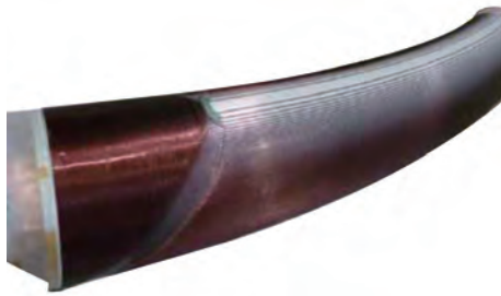
High-precision curved, saddle-shaped coil fabricated using 3D winding technology
