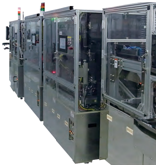
Laser welding and He sealing production line for He-filled nearline HDDs
