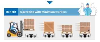
By automating the transport and rearranging of pallets in warehouses and manufacturing sites, forklift movement can be reduced. As the AMRs are able to carry heavy loads stably, safe transportation over long distances is possible. Special pallet PODs (carriers) allow direct placement of pallets on the AMR, enabling collaboration with conveyors and other robots.
