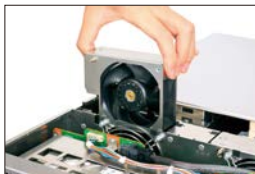
Cooling Fans replacement
