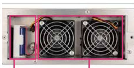
Front-end Replacement of Battery
