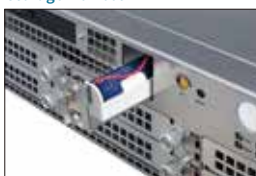
Front-end Replacement of Battery
