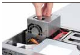
Cooling Fans replacement
