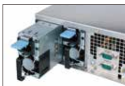
Rear-end Replacement of Power Supply Units
