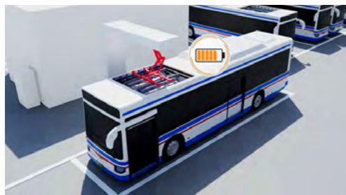
Images of EV buses with Toshiba's battery SCiB™ powered by a pantograph charging system
