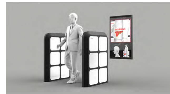
Image of the walk-through hazard detection system using millimeter-wave imaging radar
