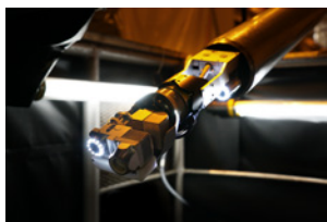
福島第一原子力発電所向け 原子炉格納容器内調査装置 Camera device for investigating inside primary containment vessel for Fukushima Daiichi Nuclear Power Plant (Courtesy of IRID)
