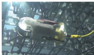
福島第一原子力発電所向け 原子炉格納容器内調査水中ロボット* Underwater robot for investigating inside primary containment vessel for Fukushima Daiichi Nuclear Power Plant *「廃炉・汚染水対策事業費補助金」により開発(IRID) Developed under "The Subsidy Project of Decommissioning and Contaminated Water Management by IRID)
