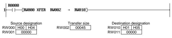
D0000 (CPU register) 45 words transfer Bank 1 F0000 (Expanded F register)
