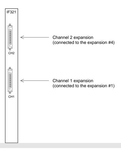
The figure below shows the T3H's maximum expansion configuration.
