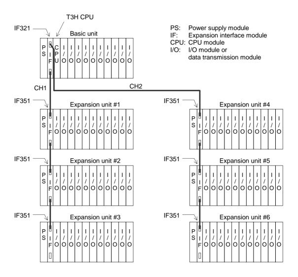
In this configuration, the T3H can handle up to 76 I/O modules. If 64 points I/O modules are mounted on all the I/O slots (76 slots), the T3H can control up to 4864 points of discrete I/O.
