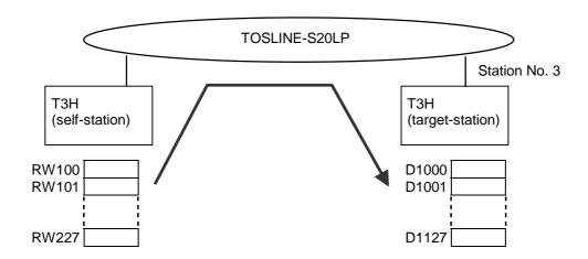
When R0020 is ON, 128 words data starting with RW100 is transferred to D1000 and after of the T3H on which station No. 3 S20LP is installed.
