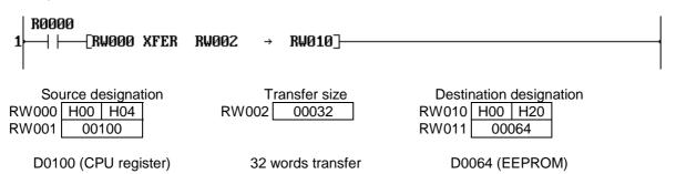
When R0000 is ON, 32 words data starting with D0100 is transferred to D0064 and after in the EEPROM. (Data write into EEPROM)
