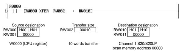
When R0000 is ON, 10 words data starting with W0000 is transferred to scan memory address 00000 and after of channel 1 S20/S20LP.
