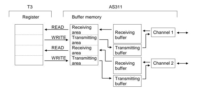
Here, a message (one set of transmission characters) means a string of ASCII characters which is ended by specified trailing code. The default setting of the trailing code is CR (carriage return code = HOD).
