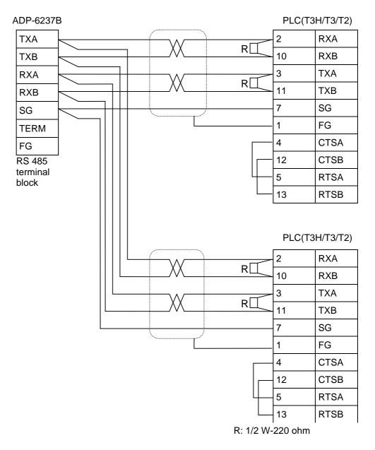
Using RS485/R232C converter (ADP-6237B):
