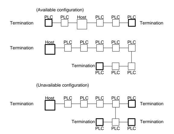
Termination resistors (1/2W-220 ohm) should be connected between TXA and TXB, and RXA and RXB, as each end of the line (termination stations).
