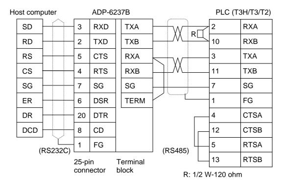
Using RS485/R232C converter (ADP-6237B):
