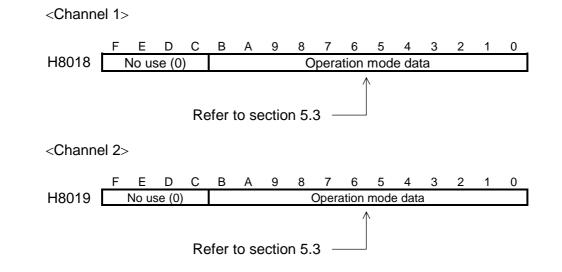
The operation mode is internally set at the timing of the gate condition is fulfilled.
