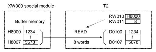
Note 1) The special module can be designated not only by the assigned register, but also by the mounting position. The mounting position is designated by a constant data for the operand A as follows.
