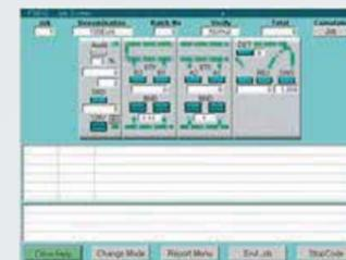
The machine has a 15-inch display. The operator sets up sorting scheme (denomination, batch size, soil level fitness, etc.) on GUI.
