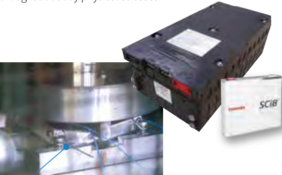
Crush Test for SCiB™ Cell Battery
