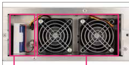
Front-end Replacement of Battery
