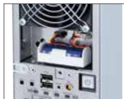
Front-end Replacement of Battery
