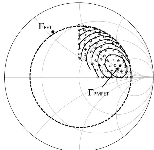
Fig. 3 Loadpull impedance of FET cell with pre-match circuit ( $\Gamma_{PMFET}$ ) and its de-embedded impedance ( $\Gamma_{FET}$ )
