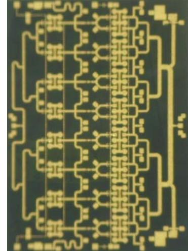
Fig. 6 Microphotograph of the developed GaN MMIC
