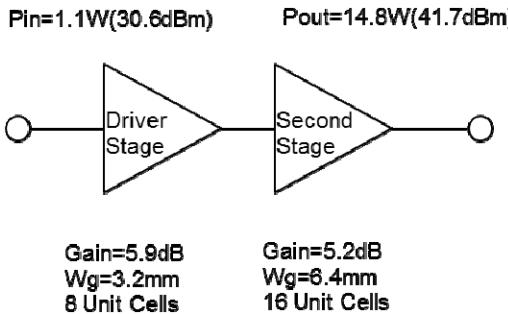
Fig.5 Block diagram of the 2-stage MMIC
