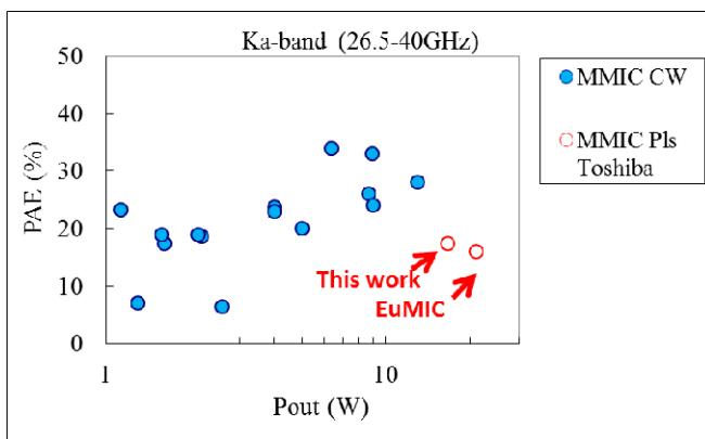
Fig. 8 PAE of GaN MMIC for Ka-band versus Pout.
