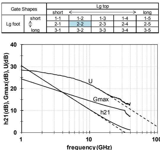
Fig. 2 h21, Gmax and Mason's U of the unit FET cells with 50μm-8-finger of Lg\_top=type2/Lg=type2
