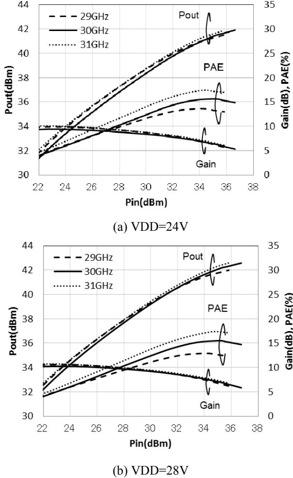
Fig. 7 Measured power, efficiency and gain with swept input power at (a) VDD=24V and (b) VDD=28V
