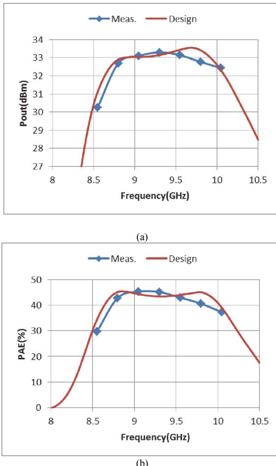
Fig. 4. Measured Pout and PAE results of 2 W X-band GaN MMIC PA with  $V_{ds} = 30$  V under pulse operation of duty of 10% and  $P_{in} = 15$  dBm. : (a) Pout; (b) PAE
