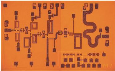
Fig. 3. Photograph of 2 W X-band GaN MMIC PA. The chip size is 2.0 mm x 3.1 mm.
