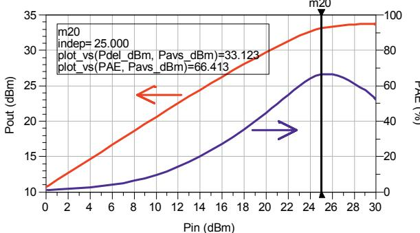
Fig. 1. Simulated output power and PAE results of a 9.3 GHz Class-F GaN HEMT unit amplifier with a Vds of 30 V.
