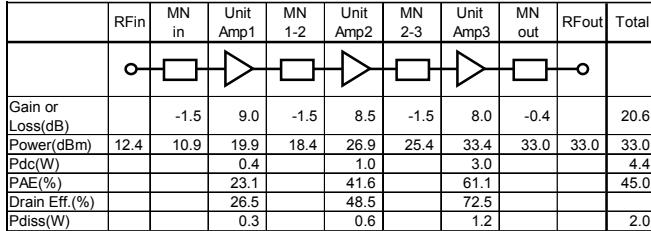
Fig. 2. A power budget for a 2W X-band GaN MMIC PA.
