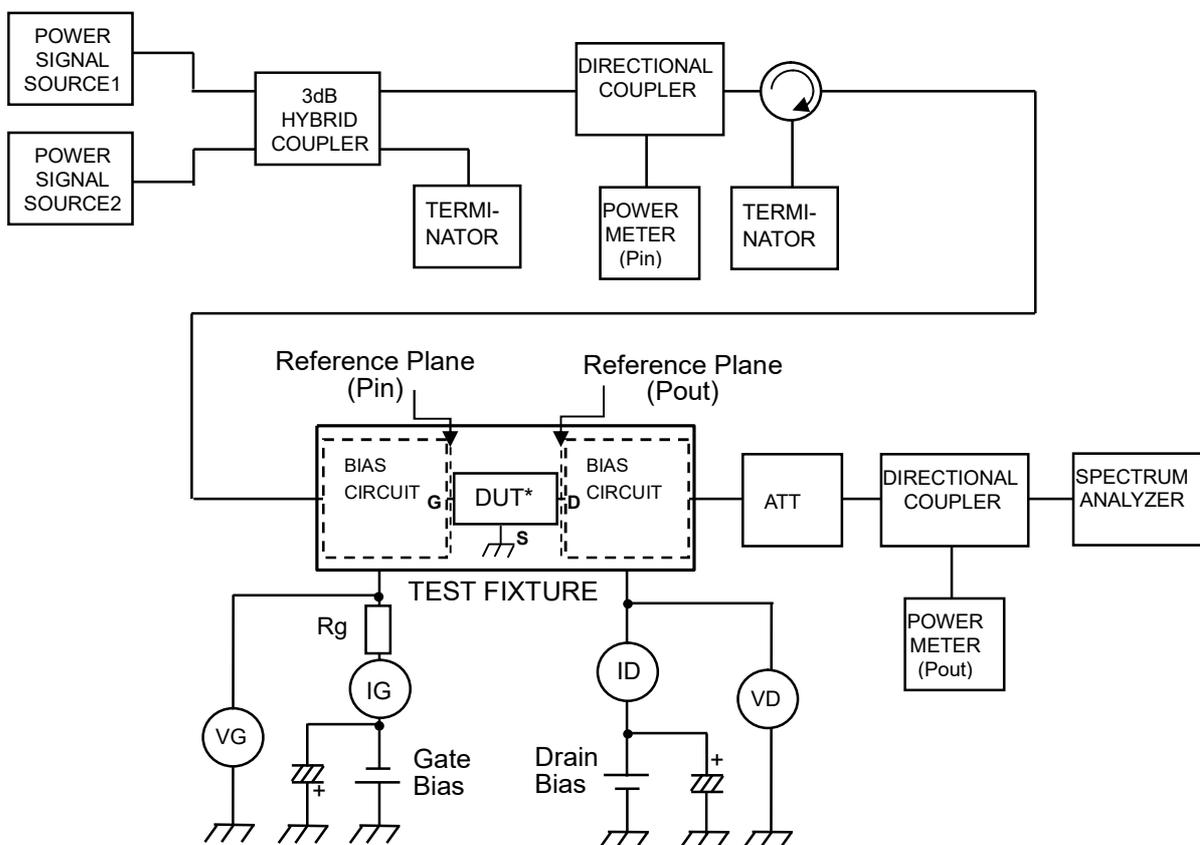
\*DUT: Device Under Test
