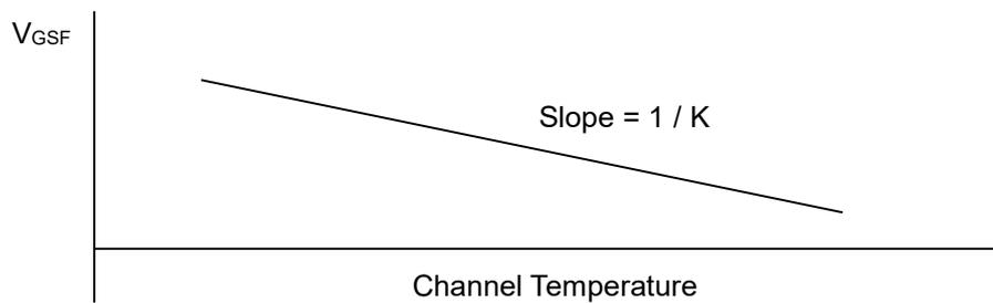
**Figure B Forward Biased Gate to Source Voltage vs. Channel Temperature**
