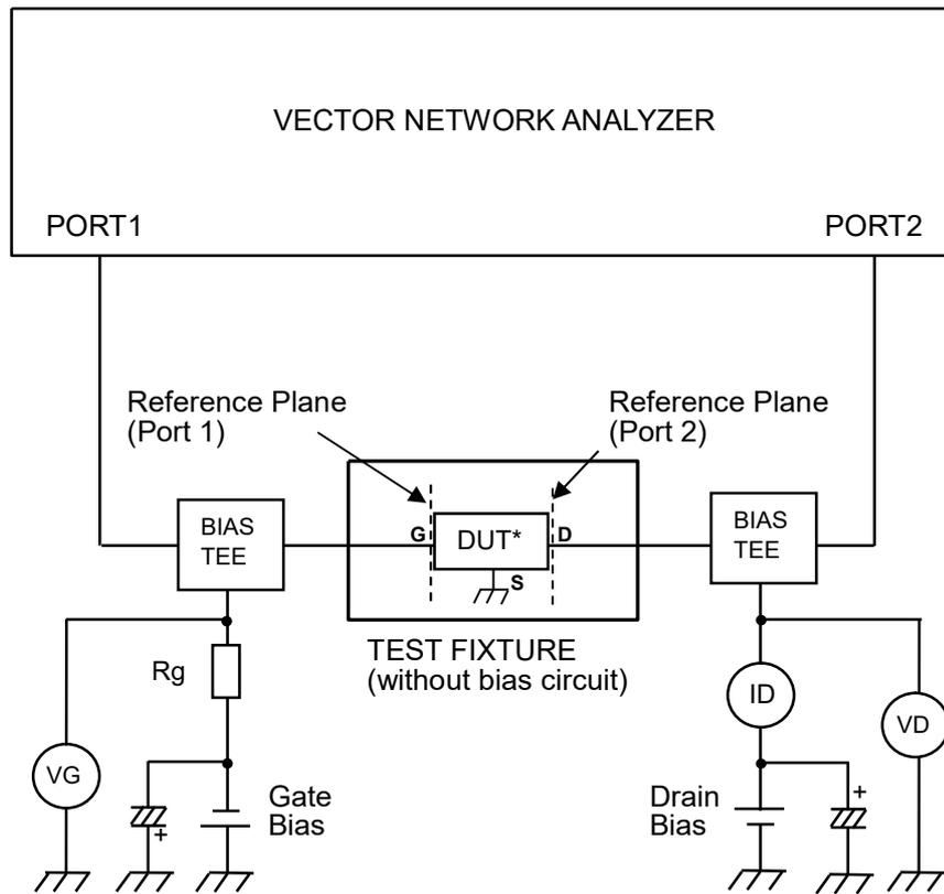
\*DUT: Device Under Test
