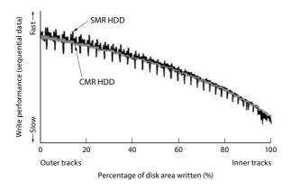
Figure 7. Comparison of sequential-write performance of CMR and SMR HDDs.
