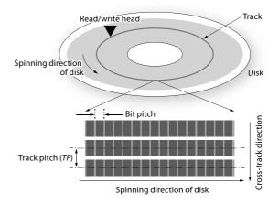
**Figure 1.** Outline of head and media of HDD. HDDs position a read/write head over a spinning disk to store and retrieve data.
