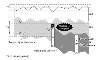
**Figure 9.** Track pitch design with emphasis on reliability. The track pitch is carefully determined to prevent accidental data erasure in the event of an external disturbance.
