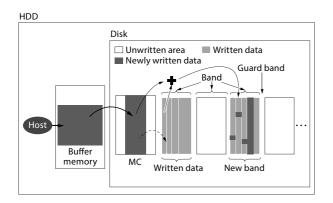
Figure 6. Data writing procedure in SMR HDD.
