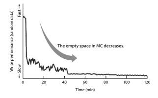
**Figure 8.** Random data writing performance of SMR HDD. The random-write performance of the SMR HDD varies, depending on the amount of free space available in the MC.
