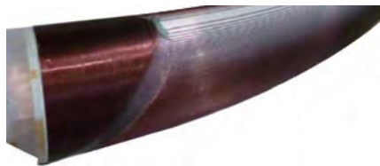
3次元巻き線機で製作した高精度湾曲くら型コイル High-precision curved, saddle-shaped coil fabricated using three-dimensional winding technology
