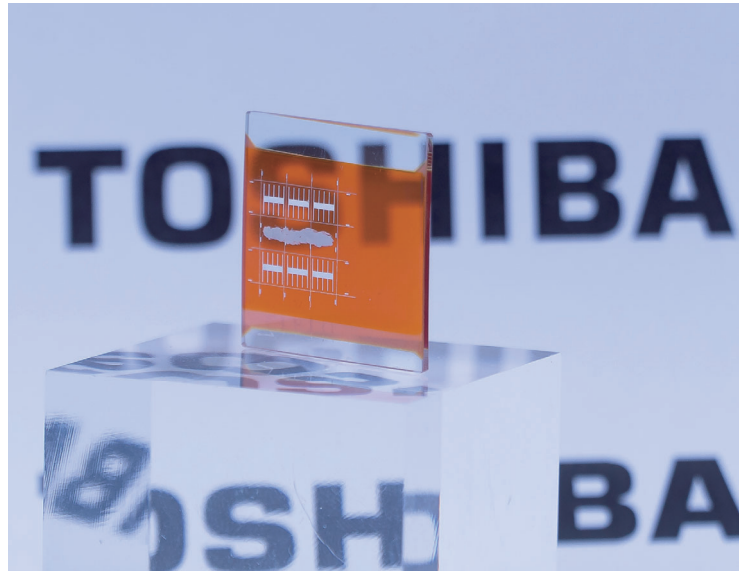
透過型Cu 2 O太陽電池 Transmission type cuprous oxide (Cu 2 O) solar cell
