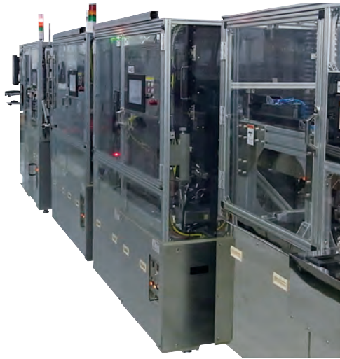
He充填HDD用レーザー溶接封止自動化ライン Laser welding and helium (He) sealing production line for He-filled hard disk drives (HDDs)
