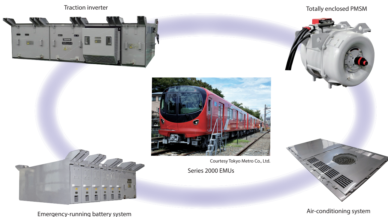
Electrical equipment for Series 2000 EMUs of Tokyo Metro Co., Ltd.
