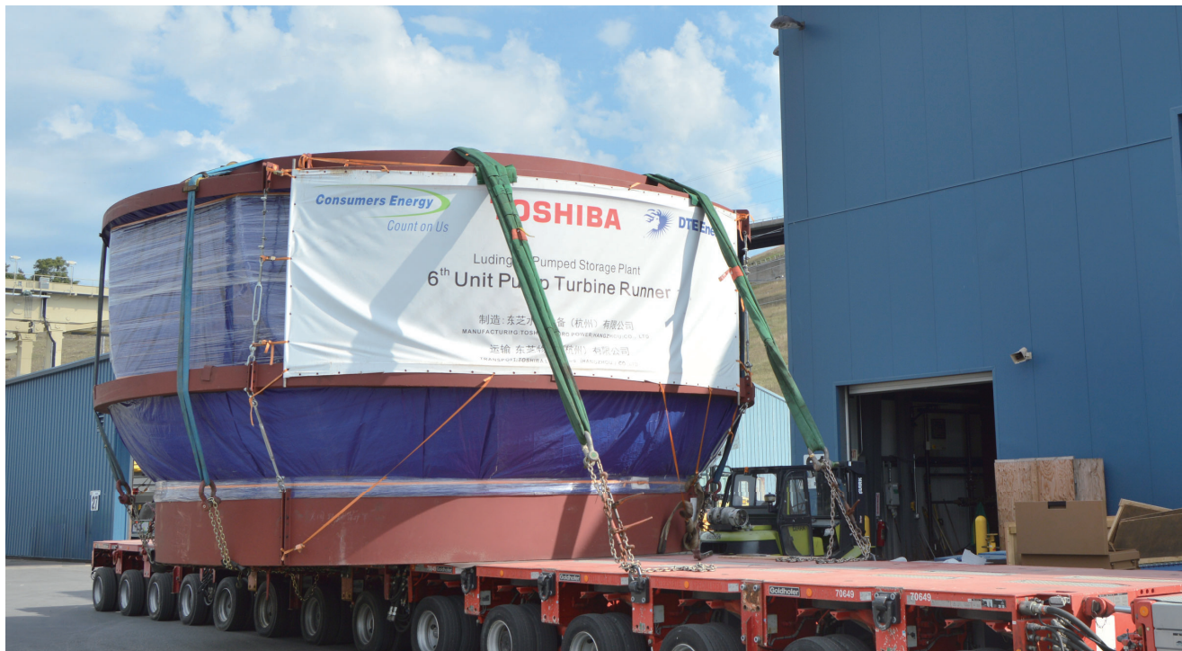
Sixth pump-turbine runner on arrival at Ludington Pumped Storage Plant
