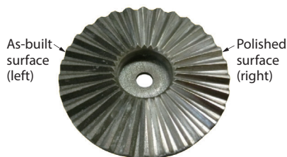
Heat dissipation part made of tungsten
