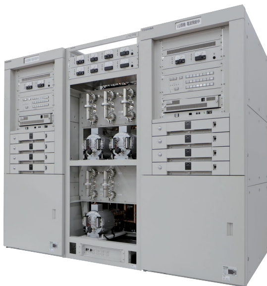
東京 芝放送所 1 kW 実験試験局用送信設備 1 kW transmitter for advanced digital terrestrial TV broadcasting installed at Shiba experimental station of Japan Broadcasting Corp.
