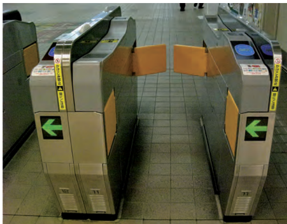
IC専用自動改札機 Standard automatic ticket gate for dedicated integrated circuit (IC) card use
