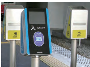
IC簡易自動改札機 Simplified automatic ticket gate for dedicated IC card use
