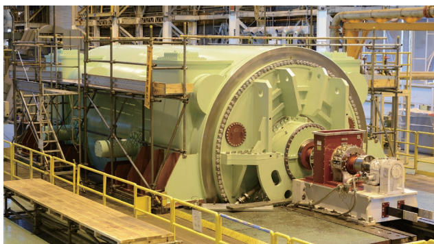
716.667 MVA 発電機の諸元と回転電気試験の様子 Specifications and scene of shop test of 716.667 MVA indirectly hydrogen-cooled generator
