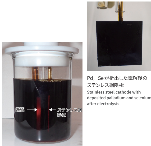
模擬高レベル放射性廃液の電解 Electrolysis of simulated high-level liquid radioactive wastes
