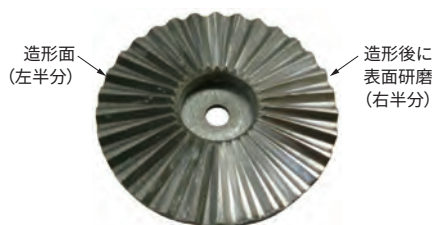
タングステン放熱用部品 Heat dissipation part made of tungsten before (left, showing as-built surface) and after being polished (right)
