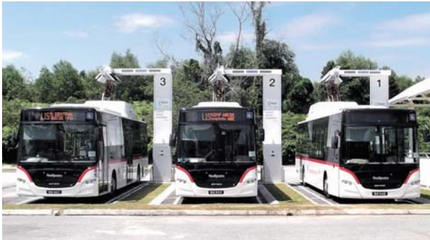
Electric buses equipped with SCiB™ lithium-ion rechargeable batteries at charging station in Putrajaya, Malaysia
