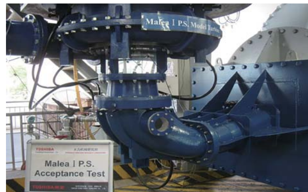
Model test of Francis turbine for Malea 1 Hydropower Plant, Indonesia
