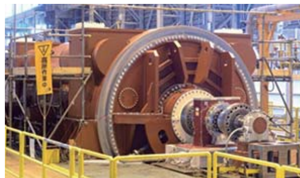
650 MVA double-end drive indirectly hydrogen-cooled generator for Ishikariwan Shinko Thermal Power Station Unit 1 of HEPCO
