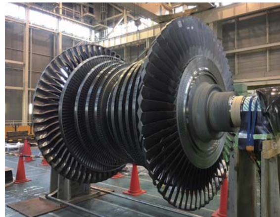
Steam turbine rotor optimized for Yanaizu-Nishiyama Geothermal Power Station of Tohoku Electric Power Co., Inc.
