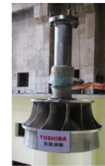
Turbine runner with shaft
