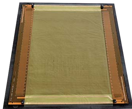
宇宙用ダストセンサー用FPC Flexible printed circuit (FPC) board for measuring size of space debris
