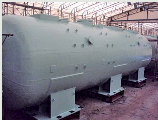
Underground light-oil storage tank for emergency diesel generators of nuclear power plants
