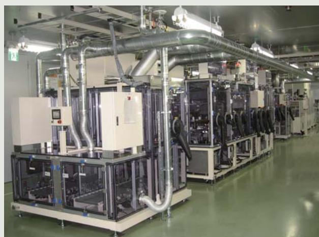
Liquid injecting and sealing machine for 10 Ah/20 Ah SCiB™ battery cells
