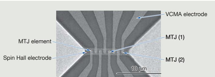
(a) Scanning electron microscope (SEM) image of fabricated VoCSM prototype structure with eight MTJs
