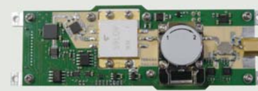
Compact high-power generator for portable microwave surgical instruments
