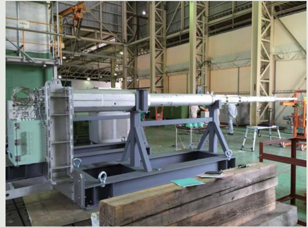
Heat-thermo type spent fuel pool water level and temperature measurement sensor
