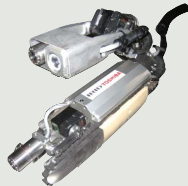
Remote-controlled robot for internal PCV investigation
