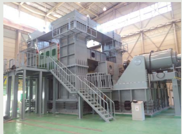
Full-scale seismic isolator break test machine
