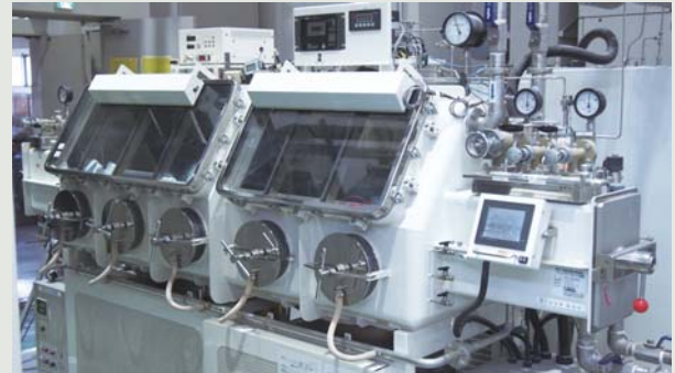
Molten salt electrorefining test equipment to recover long-lived radionuclides
