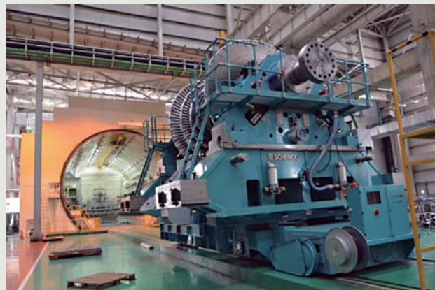
High-speed balancing test equipment and steam turbine rotor for Kudgi Super Thermal Power Plant Unit 2, India
