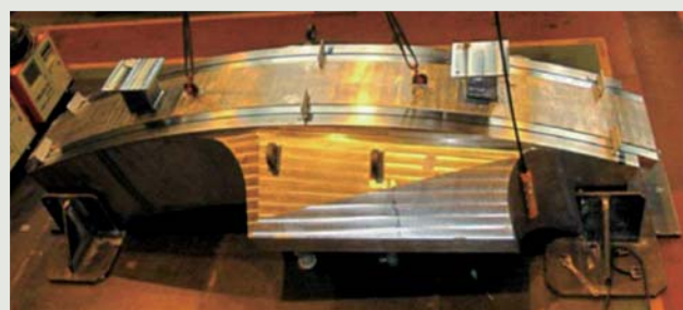
Manufacturing of TF coil winding (upper) and structure segment (lower)
