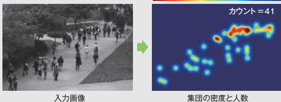
▲ 群衆を撮影したカメラ画像を用いた集団の密度と人数の推定 Estimation of density and number of people included in crowd based on image data obtained by camera
